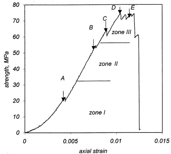
Fig. 2. Stress–strain curve of a rhyolite sample. Arrows on the graph show moment of EMR pulse excitation. Zone I is defined by individual pulses; Zone II is characterized by pulses with uneven shape and/or groups of pulses; Zone III shows particularly lengthy pulses (see elaboration of significance of arrows A–E in Rabinovitch et al., 1996).
