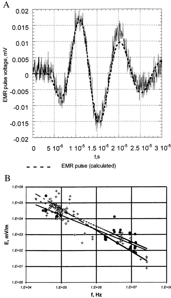
Fig. 3. A) An experimental EMR pulse and its numerical fit; B) Amplitude–frequency relation of EMR pulses associated with chalk, granite and glass-ceramic compression (• chalk; ◊ granite; + glass-ceramic; — chalk trendline; --- granite trendline; —·— glass-ceramic trendline).
