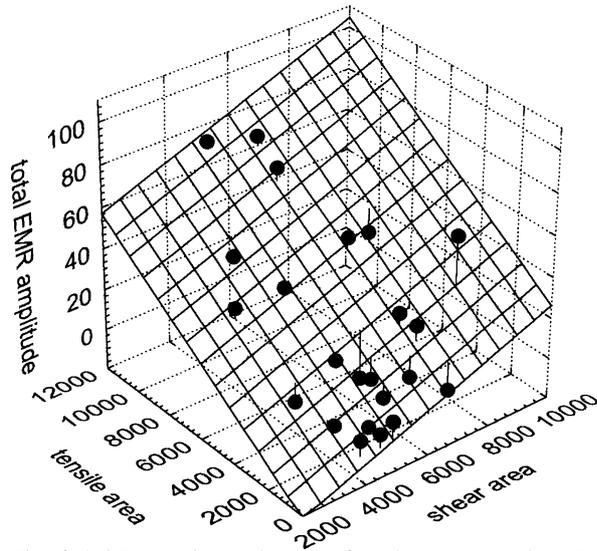
Fig. 6. A 3D experimental graph of total compensated EMR pulse amplitudes (V/m) versus total areas (mm<sup>2</sup>) of tensile and shear crack areas of all investigated samples and their fit.
