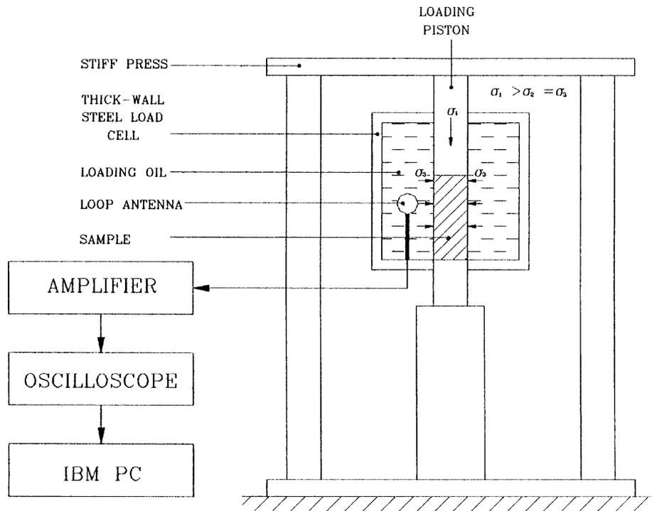
Fig. 1. Schematic diagram of experimental arrangement for measuring EMR of rock fracture.
