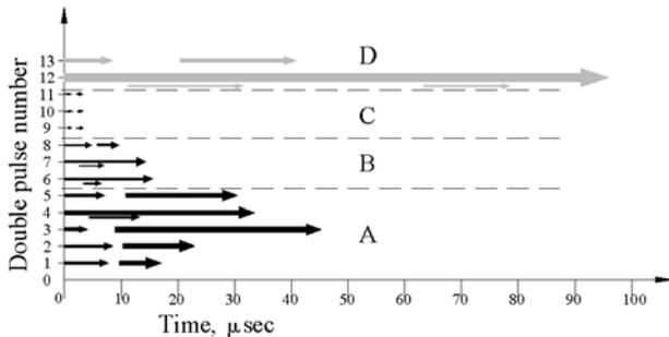
**Figure 9.** Description of all double pulses observed in chalk: each double pulse is shown by two black arrows corresponding to the single pulses constituting the double pulse; dashed horizontal lines separate the pulses emitted by different chalk samples denoted by (A)–(C). Triple and double pulses emitted by glass ceramics (see also figures 5 and 7) are also shown for comparison by grey arrows (D).
