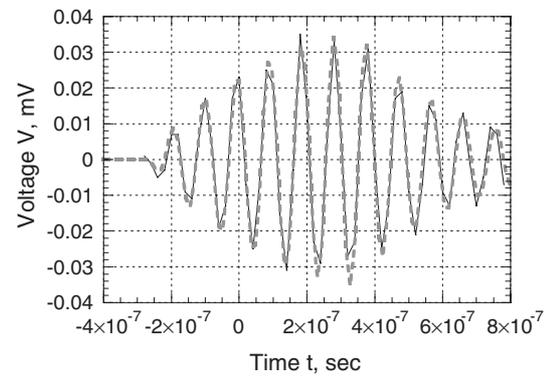
**Figure 1.** Experimental EMR pulse emitted from chalk with the following fitted parameters:  $A_0 = 0.041 \pm 0.002 \text{ mV}$ ,  $\tau = 3 \times 10^{-7} \pm 0.27 \times 10^{-8} \text{ s}$ ,  $t_0 = -2.683 \times 10^{-7} \pm 9 \times 10^{-10} \text{ s}$ ,  $T = 3.4 \times 10^{-7} \pm 2 \times 10^{-8} \text{ s}$ ,  $\omega = 6.59 \times 10^7 \pm 1 \times 10^5 \text{ s}^{-1}$ .
