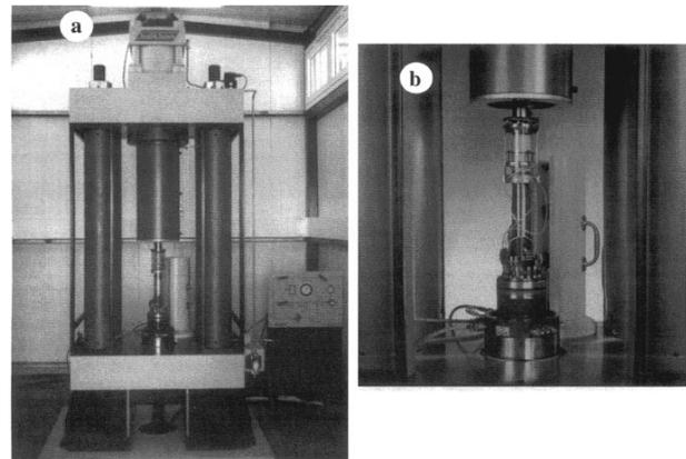
**Figure 2.** Compression press: (a) the triaxial load frame, (b) the sample stack.
