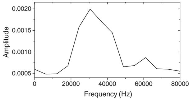
**Figure 3.** An example of frequency spectrum of a double pulse.
