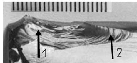
**Figure 8.** Photograph of the crack in glass ceramics which emitted the double pulse shown in figure 7.
