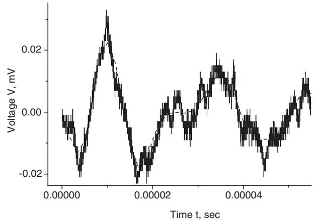
**Figure 7.** Double pulse emitted by a stress-relaxation crack in glass ceramics; its fitting parameters are:  $T'_1 = 84.6 \mu\text{s}$ ,  $\omega_1 = 4.22 \times 10^5 \text{ s}^{-1}$ , corresponding to the earlier, smaller crack, and  $T'_2 = 20.4 \mu\text{s}$ ,  $\omega_2 = 3.39 \times 10^5 \text{ s}^{-1}$ , which corresponds to the larger crack.
