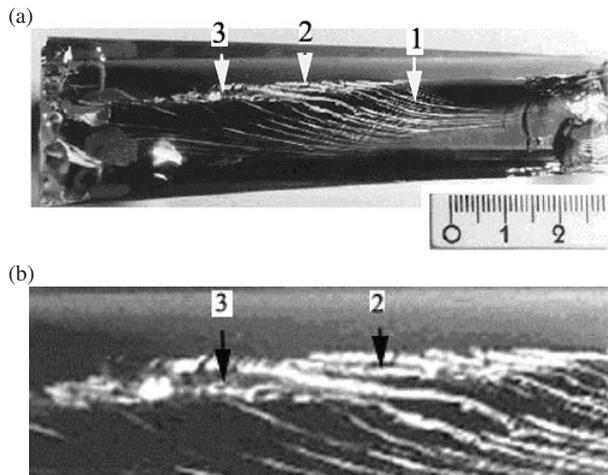
**Figure 6.** (a) Photograph of the crack in glass ceramics which emitted the triple pulse shown in figure 5. Initial striae on the main crack are marked by 1 and the striae continuations by 2 and 3. (b) Enlarged view of the two striae continuations. The striae continuations are misaligned with respect to the initial striae, and therefore the distinction of 2 and 3 is not very clear.
