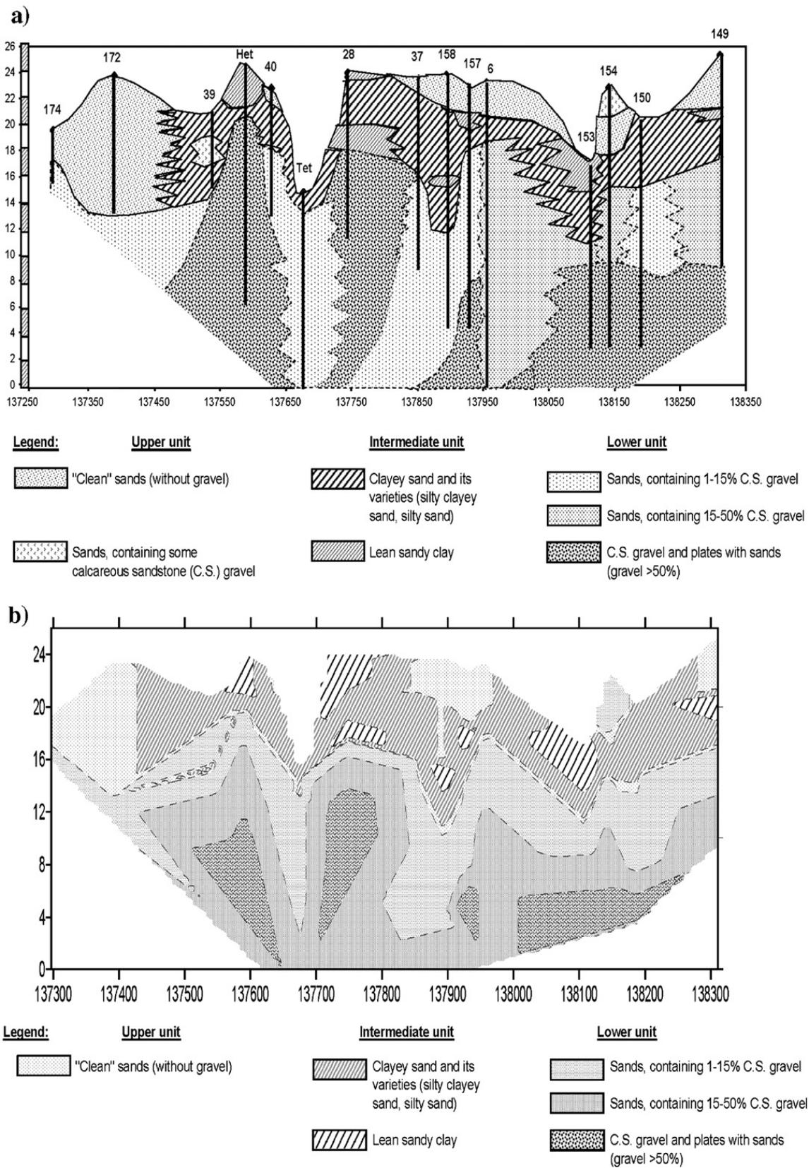
Fig. 1a. Hand drawn vertical section of the rear site of Ashdod Port. Numbers and black lines show numbers and depths of boreholes. b. Computer made vertical section of the same site as in a. Both vertical sections are drawn in the same scale, though their horizontal scale is different from their vertical scale.
