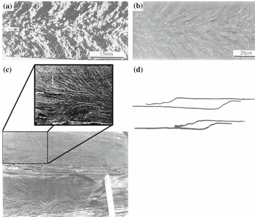
**Fig. 1** (a) Chevron pattern in low-alloy steel (from Hull 1999, p. 9). (b) Chevron pattern in silica-based-sol-gel (from Hull 1999, p. 9). (c) Two plumes decorating joints that cut Devonian siltstone from the Appalachian Plateau, N.Y., propagating towards left. The ruler length is 20 cm. Frame of inset is marked (from Bahat and Engelder 1984). *Inset in c.* A magnified part of Fig. 1c, showing alternating radial zones of dark tensile valleys
