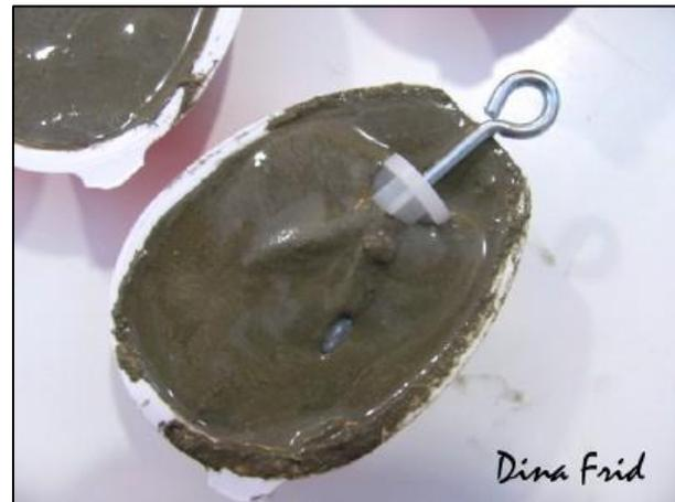
Dissolve cement quite following to the instructions on its package while adding slightly more water than it is recommended to get the cement slurry to be liquid.
