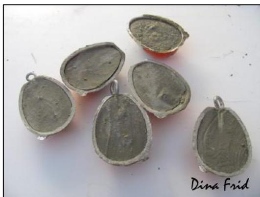
The next day, pull the concrete blanks out of the plastic shells. Providing the concrete is hard, the blanks can be easily pulled out.
