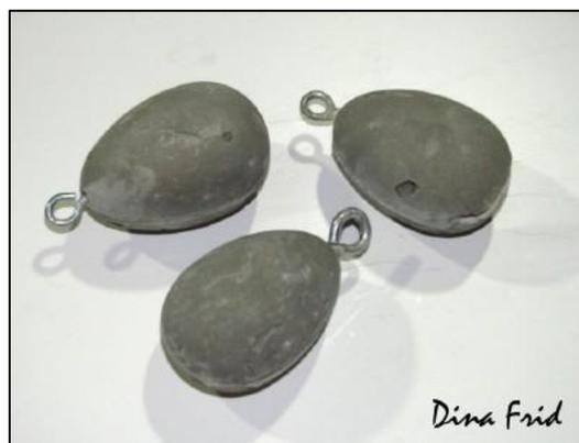
Prepare just a little cement as before and spread it over both halves of the blanks and glue them. If the surface of the blanks is covered with air holes, spread the slurry on them too. Leave the blanks for the day for drying.
